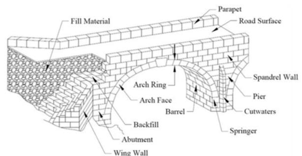
Figure 1: Overview of typical terminology for masonry arch bridges [1].
