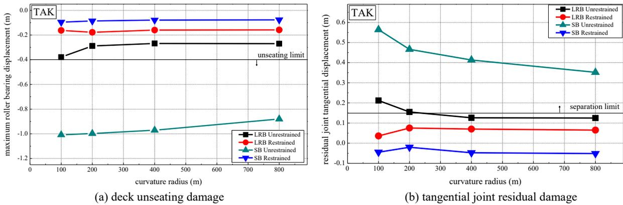
Fig. 3 Effect of seismic isolation and unseating prevention cables on seismic damage
