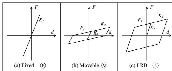
Fig. 2 Analytical models of bearing supports
