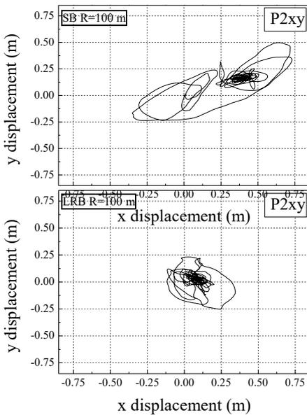
Fig. 4 Effect of seismic isolation on pier top damage from TAK
