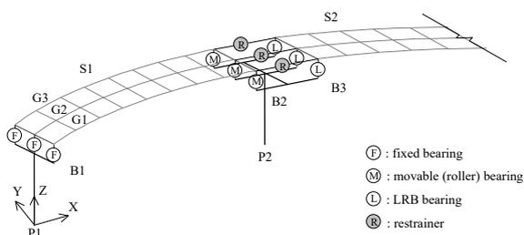
Fig. 1 Detail of viaduct finite element model
