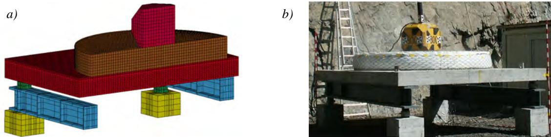
Fig. 1: Finite element model a) and experimental setup b) of a large scale test
