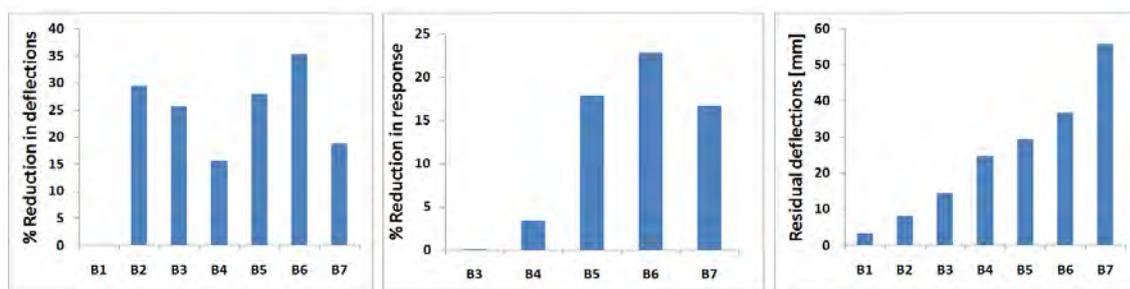
Fig. 2: Reduction in deflection and response of slab due to consecutive loading
